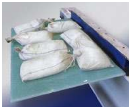
Laminated safety glass consisting of TROSIFOL® ES between two plies of fully tempered glass
